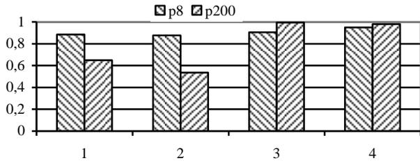
Figure 7. Probability of changes in voltage magnitudes at nodes 8 and 200 for the initial operating conditions (1), operating conditions after the reinforcement of weak ties (2), operating conditions after the implementation of control actions (3), and operating conditions under simultaneous implementation of control actions and reinforcement of weak ties (4)
