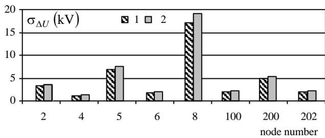
Figure 2 Mean square deviation of voltage magnitudes at the nodes of the test scheme obtained by the linear method – 1, the Monte Carlo method – 2
