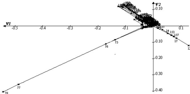
Figure 8. Projection of the real network graph on the plan in coordinates of the first ( $v_1$ ) and second ( $v_2$ ) right singular vectors that correspond to voltage magnitudes
