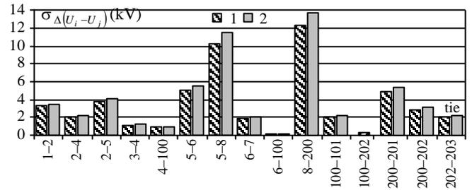
Figure 5. Mean square deviations of voltage magnitude differences in the ties of the scheme obtained by the linear method – 1, the Monte Carlo method – 2
