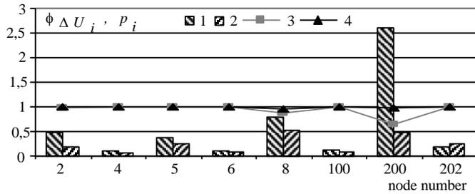
Figure 4. Values of  $\phi_{\Delta U_i}$  – 1, 2 and probability  $p_i$  that voltage magnitudes are within the feasible limits – 3, 4, for the initial operating conditions 1, 3 and the conditions obtained as a result of the network reinforcement and selection of control actions 2, 4
