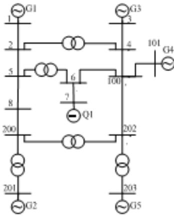
Figure 1 Scheme of a 14-node test network
